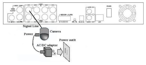
DVR-400 provides 4 x BNC connectors for video source input.
